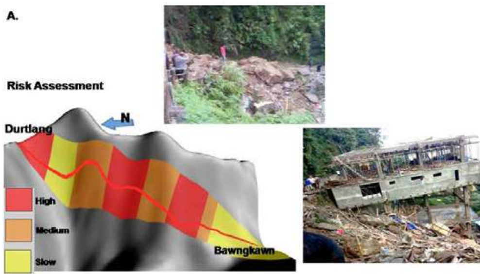
Figure 4: Risk Assessment for the Aizawl-Durtlang Road section. (A) Probable risk zones in the thematic layer map and some recent rockfall events in the area & (B) The Layer is superimposed in Google Earth image to understand most hazardous sections of the road. It also includes the wedge failure streoplot for different sections which imply the rock fall and slide probability.
